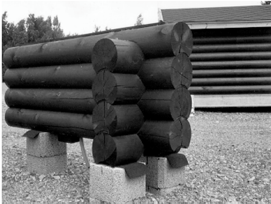
Figure 1-Test set-up for testing the moisture behaviour of log buildings in field conditions. In the foreground, test rail for the systematic part of study; in the background, a test cabin.
