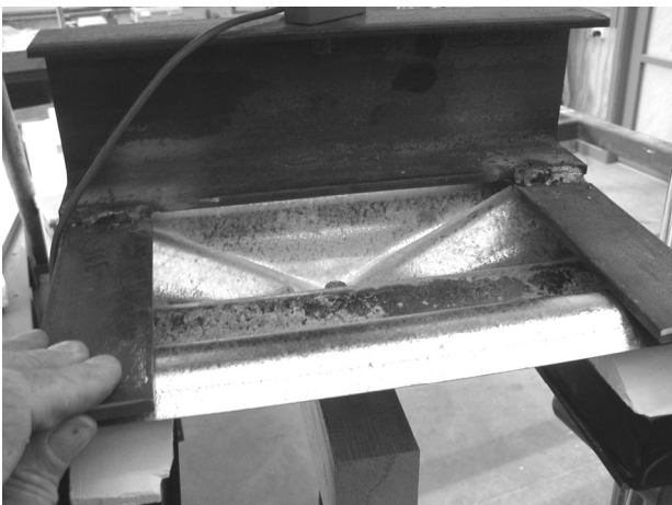
Figure 3. Roof fixings test specimen for the Probabilistic Approach to Determining the Effects of Wind on Buildings project.
