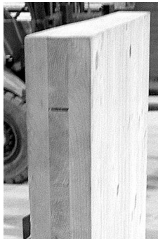
Figure 1. Detail of cross-laminated board.(Middle board has tension rings running in opposite direction to outside two boards)
