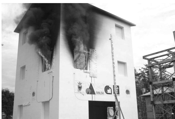
Figure 5. Three storey cross-laminated building fire tested after the earthquake tests.
