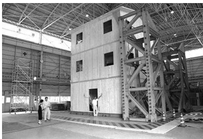
Figure 4. Three storey cross-laminated building tested on second largest shake table in Tsukuba Japan.
