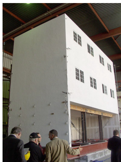
Figure 1: Test building on shaking table
