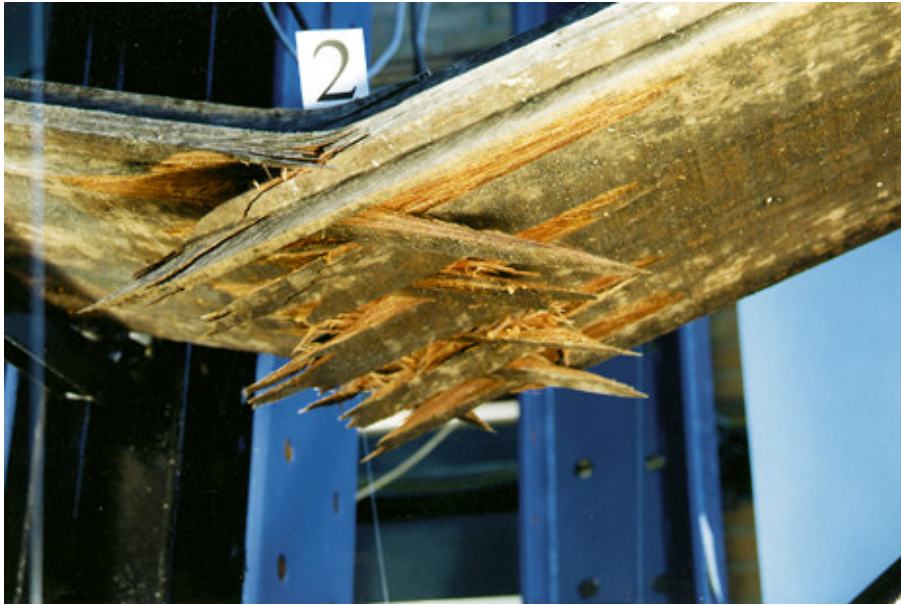
Figure 3 - Typical failure pattern of azobé boards.
