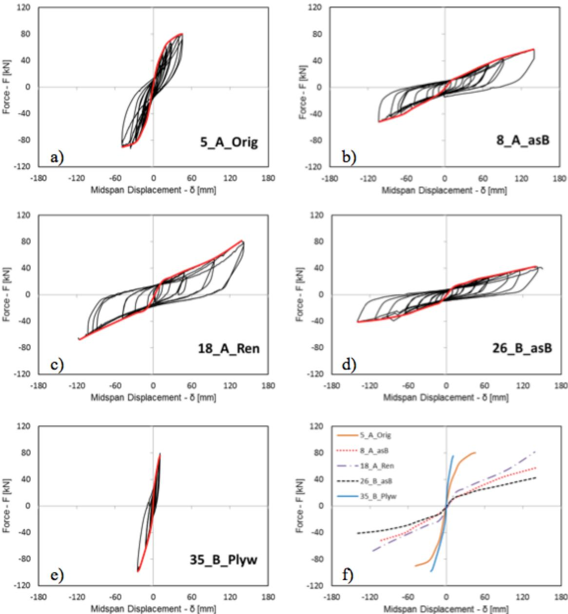
Fig. 5 Cyclic tests: a) specimen A - original condition (with ceiling and metal sheathing); b) specimen A - as-built; c) specimen A - re-nailed; d) specimen B - as-built; e) specimen B - retrofitted with a plywood panel overlay; f) backbone curves
