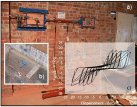
Fig. 2 New shear transferring anchoring system: a) anchor test setup; b) new anchor installation; c) cyclic test results
