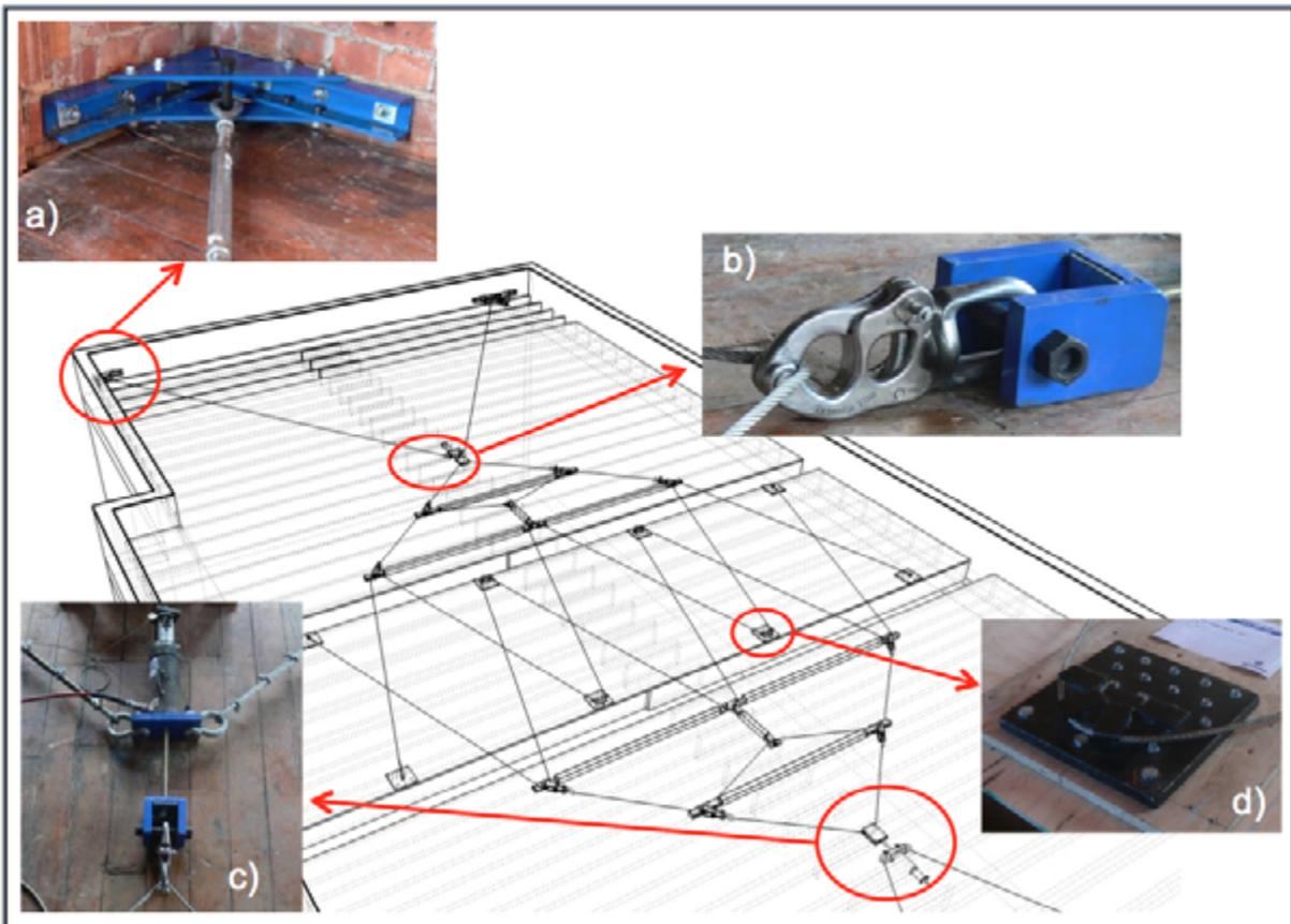
Fig. 3 Details: a) wall connection bracket; b) snap shackle for instantaneous load-release; c) hydraulic actuator; d) central loading plate
