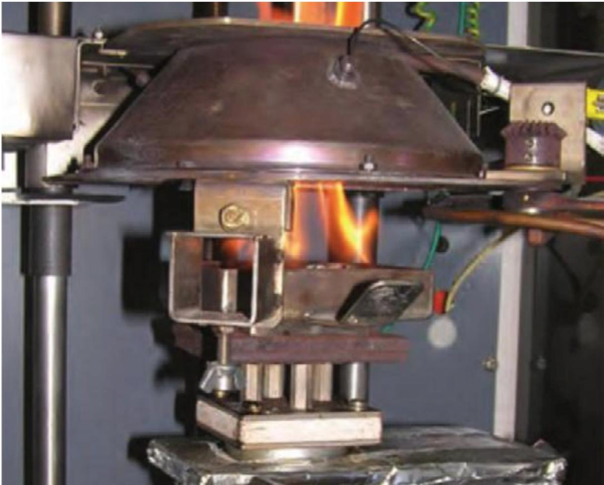
**Figure 2:** A 100mm x 100mm sample burning in the cone calorimeter test, ISO 5660 or AS/NZS3837 (Whiting 2012).
