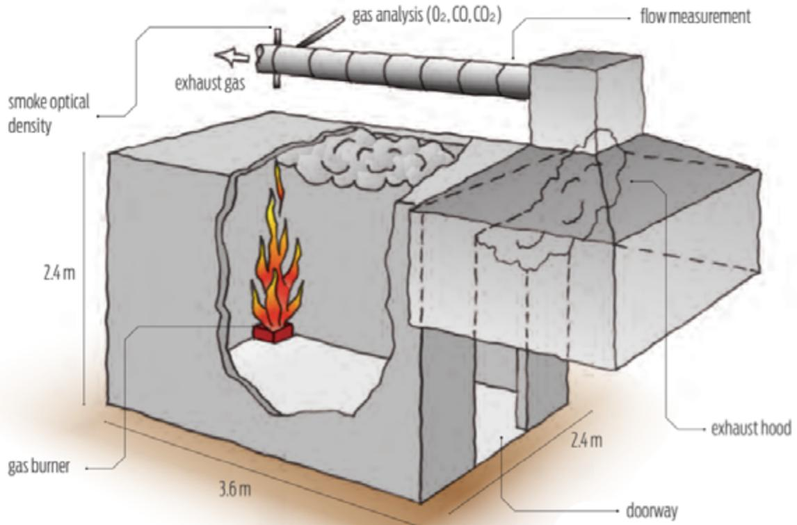
Figure 1: Full-scale ISO 9705 test.
