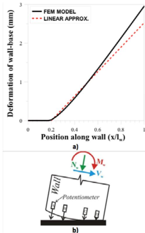
Figure 5: Displacement profile at the base of the walls a) Example FEM model b) Diagram with potentiometers
