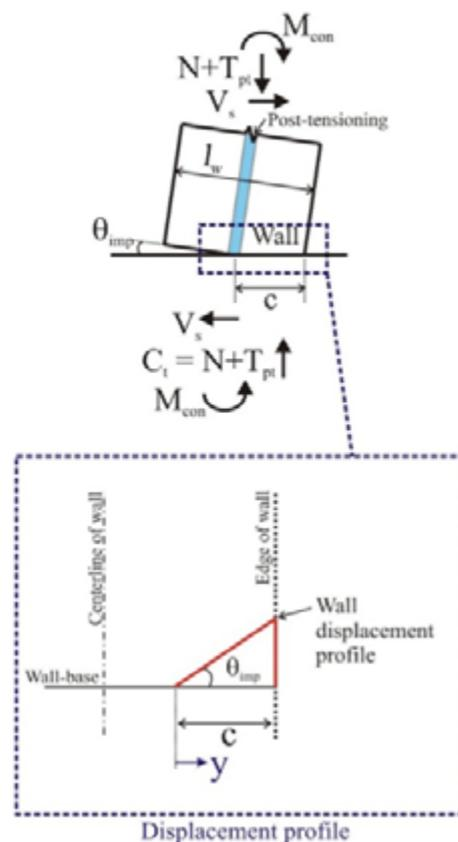
Figure 1: Rocking post-tensioned timber wall equilibrium condition and connection deformation
