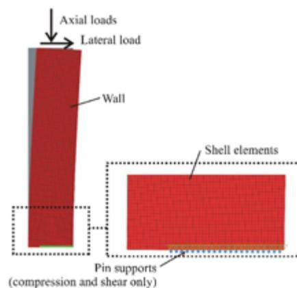
Figure 2: Boundary conditions and applied loads for the benchmark FEM of the wall
