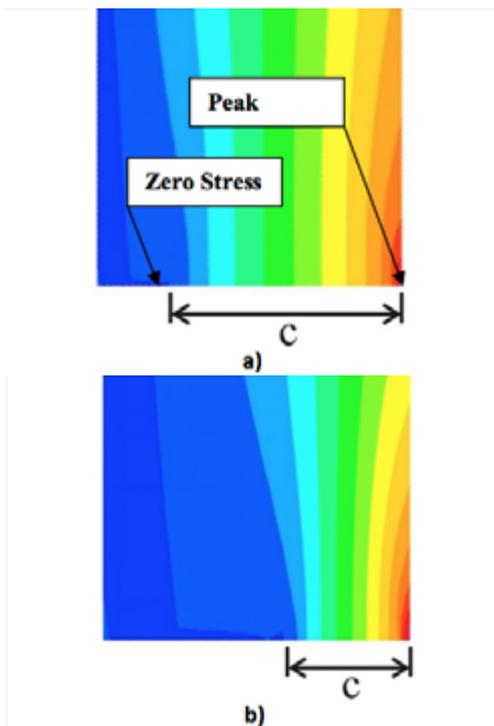
Figure 3: Longitudinal stresses at the base of the wall: a)  $c/l_w = 0.75$  b)  $c/l_w = 0.41$
