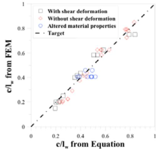
Figure 4: Correlation between the predicted and FEM neutral axis depth
