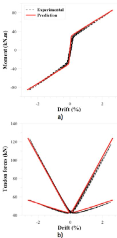
**Figure 6:** Experimental - analytical comparison for Subassembly: a) Connection moment b) Tendon forces c) Neutral axis depth d) Observed neutral axis depth at 2.5% drift
