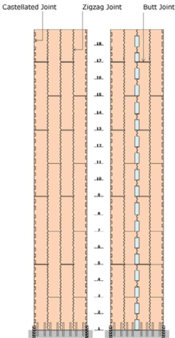
**Figure 5:** Eighteen level Integrated Panel Core - Side and End Elevations. Foundation attachments shown - hold down connections, and cantilever steel members (at corners)
