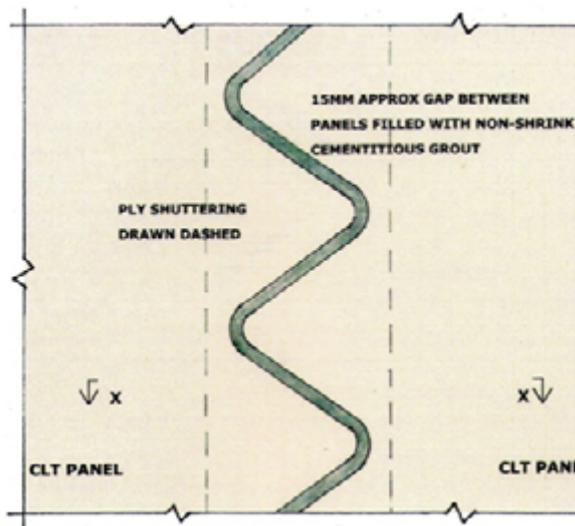
Figure 8: Elevation of zigzag joint for external walls of the central core
