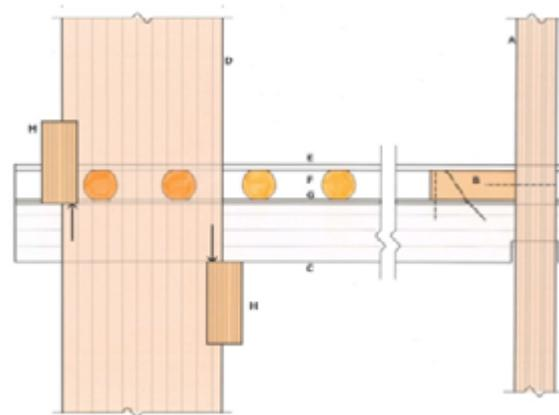
**Figure 11:** Floor Beam Elevation (section z on Figure 3), A - core wall, B - ‘hoop’ beam (Screw fixings to core and floor beams are indicated), C - engineered timber floor beam, D - engineered timber column, E - flooring, F - pole floor joists, G - ceiling, H - corbels to transmit beam moments to the column
