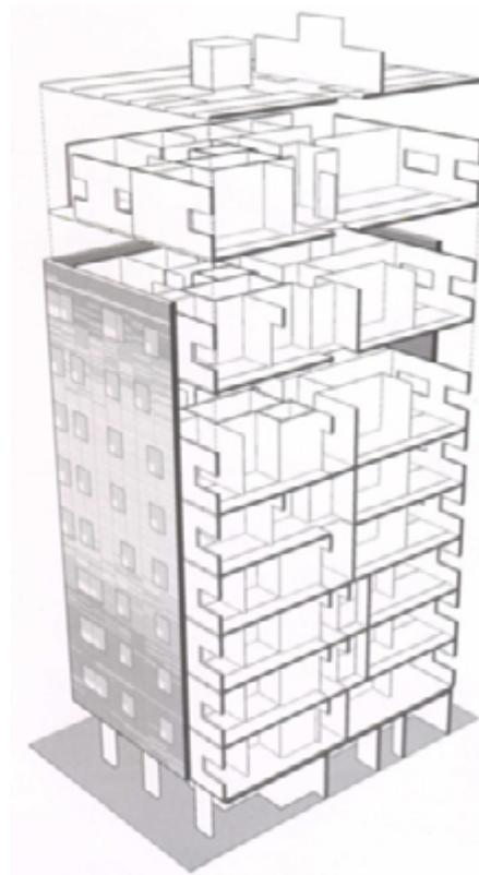
**Figure 13:** Isometric of Stadthaus Building, London, showing the close spaced CLT walls
