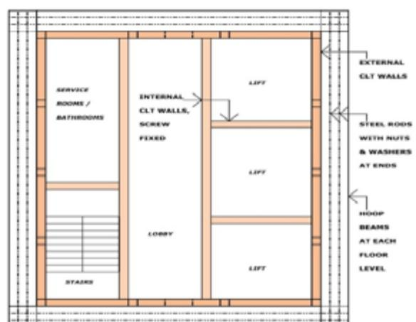
Figure 4: Plan of internal walls and architectural functions of the integrated panel core. Timber hoop beams are shown including the internal steel rods
