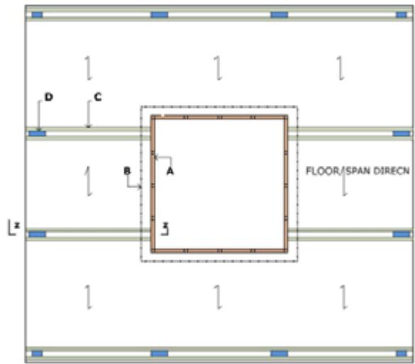
Figure 3: Plan of structure, A - integrated panel core, B - 'hoop' beam at each floor level, C - engineered timber floor beam, D - engineered timber column
