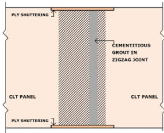
Figure 9: Section (X-X on figure 8) of zigzag joint for external walls of the central core
