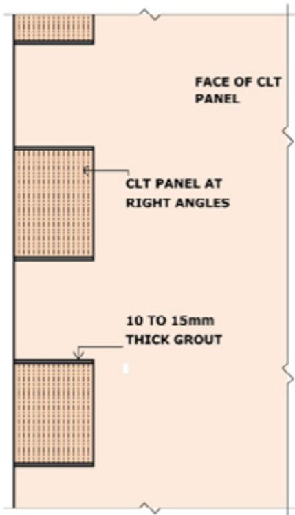
Figure 7: Elevation of castellated joints at the corners of the central core (the notches' depth is the same as the panel thickness)
