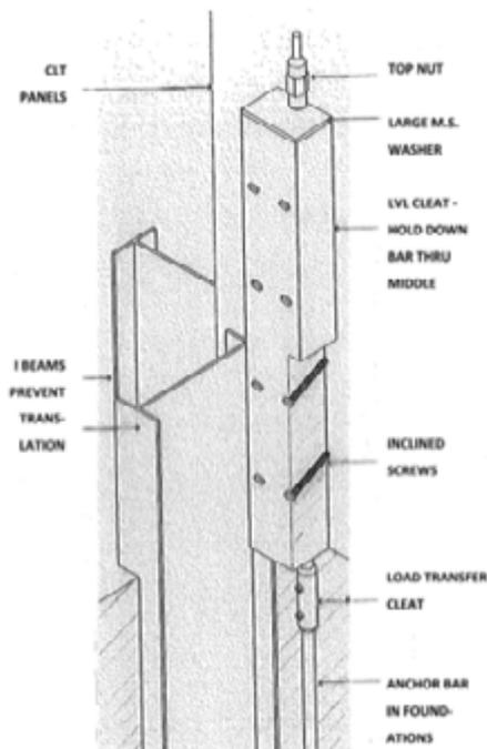
**Figure 10:** Diagrammatic isometric of a corner of the core to foundation connection showing pairs of steel members at corners to prevent core translation, and one of the vertical hold-down bar arrangements. (LVL Cleat cut-away for clarity)
