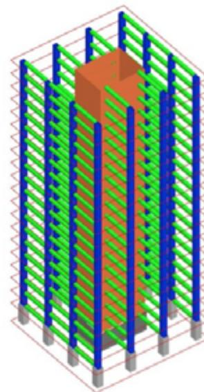
**Figure 1:** Isometric of proposed timber structural system for twenty storey building with a rectangular core of integrated CLT panels, and engineered timber columns & floor beams
