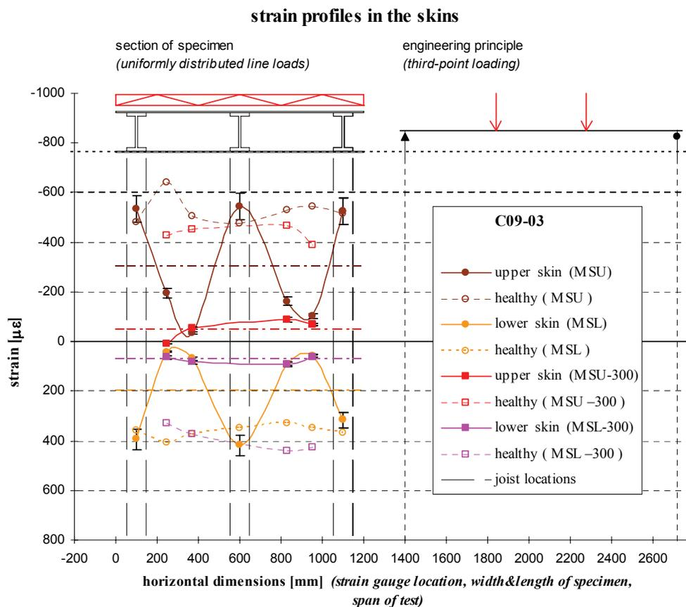
NOTE: the dashed curves with markers depict the strain profiles of the healthy-state specimen – data calibrated to the load intensity of the specimen in damaged state.
