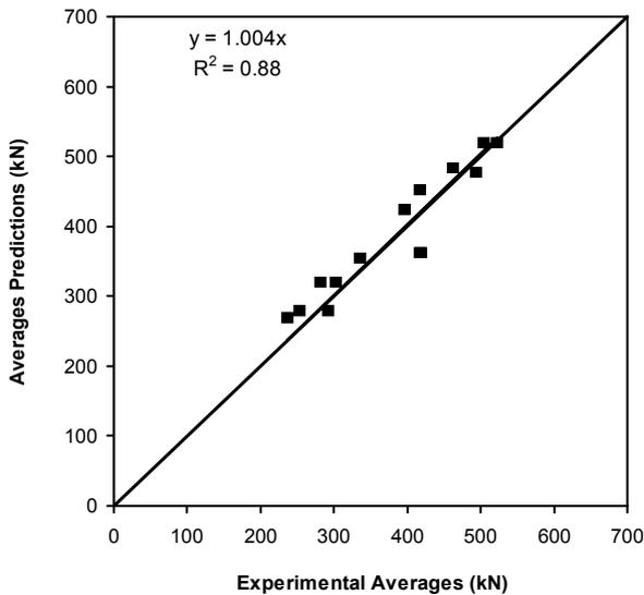
Figure 5. Predicted averages of connection capacity vs. experimental resistance averages in group tear-out failure mode
