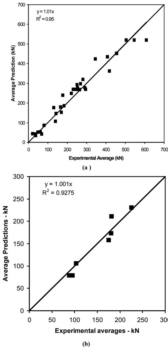
Figure 4. Predicted averages of connection capacity vs. experimental resistance average in row shear failure mode (a) steel-wood-steel connections (b) wood-steel-wood connections
