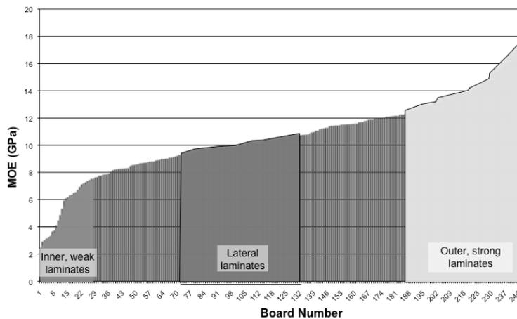
**Figure 4. Selection of boards for 100 x 21 mm panels**
