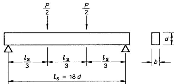
Figure 2. Testing configuration for bending and MOE testing (AS/NZS 4063) [15]
