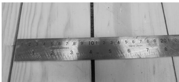
Figure 3. Gaps between outer boards after fabrication
