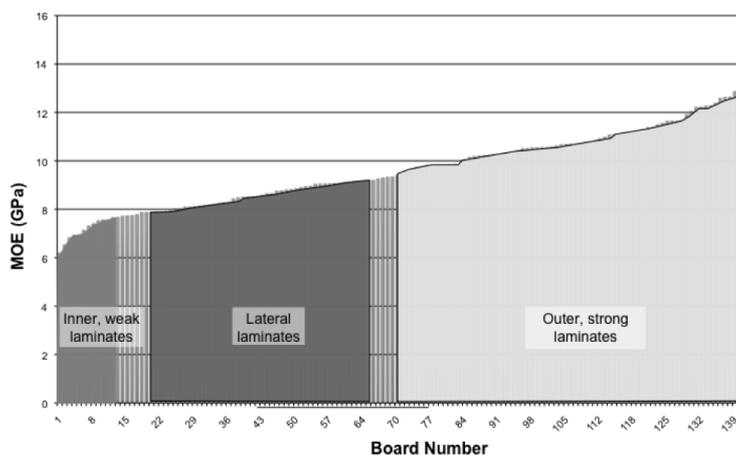
**Figure 5. Selection of boards for 90 x 41 mm panels**
