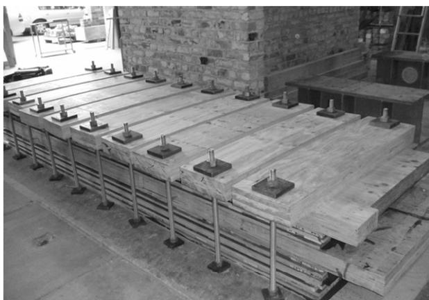
Figure 1. Press with three CLT panels curing
