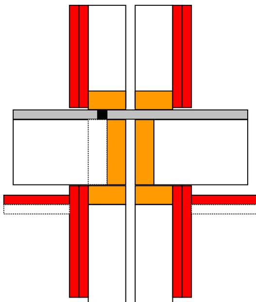
The second detail is for a single frame and resilient rail inter-tenancy wall requiring structural connection at floor level. Again the particle board is carried through the cavity, and cut and filled with an acoustic sealant on one side of the assembly.
