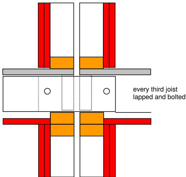
Despite the structural connection between joists, testing between bedrooms gave field results FSTC 55 (-2dB), FSTC 52 (-5dB) and FSTC 47 (-10dB). The results measured diagonally between bedrooms and the kitchen / lounge areas were FSTC 58 (+1dB) and FSTC61 (+4dB) and FIIC 74.
