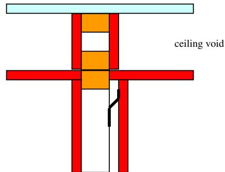
Field testing recorded FSTC 46 (-9dB) between units. Five switch boxes (some back to back) and an intercom unit penetrated the wall. The last item appeared to be a significant airborne flanking path. The wall to ceiling detail was also identified as a structure borne flanking path. Fixing the ceiling lining on a resilient clip and batten system would have eliminated this flanking path.
