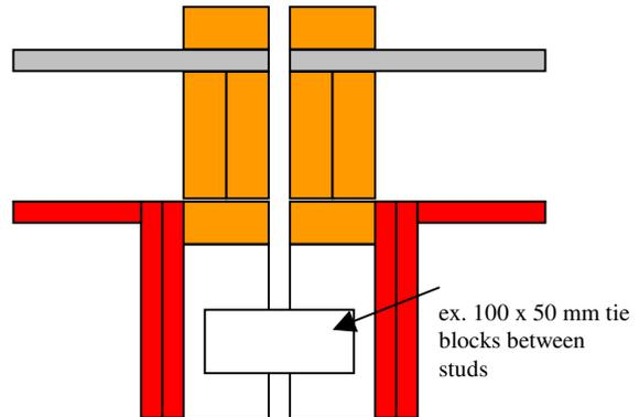
Structural tie blocks were used in some locations. Testing between apartments with tie blocks gave field results between the lounge areas of FSTC 53 (-3dB) and FIIC 63. Without tie blocks these results were FSTC 56 (-1dB) and FIIC 66. Testing between a lounge and downstairs bedroom was only carried out where tie blocks were present and gave FIIC 70.
