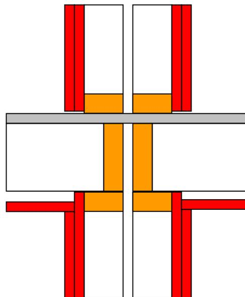
The inter-tenancy walls consist of double ex. 100 x 50 mm timber frames separated by 50 mm. R 1.6 polyester blanket was placed in the cavity. The walls are lined each side with a layer of 12.5 mm Gib® Fyrelite over 9.5 mm Gib® Fyrelite. No test data exists for this construction, but acoustic consultants Marshall Day Acoustics estimated the laboratory performance as STC 60.
