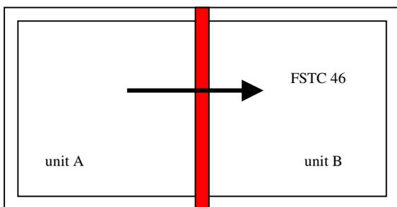
The inter-tenancy sound control wall system consists of a single ex. 100 x 50 mm timber frame with a resilient rail to one side and R1.8 glass fibre cavity insulation. The wall was lined on both sides with 2 layers of 12.5 mm Gib® Fyreline. This Gib® System GBT(L)A 90r has a published laboratory performance of STC 55.
