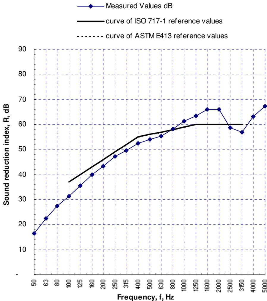
Figure 2: Determining STC rating by fitting the standard curve test results
