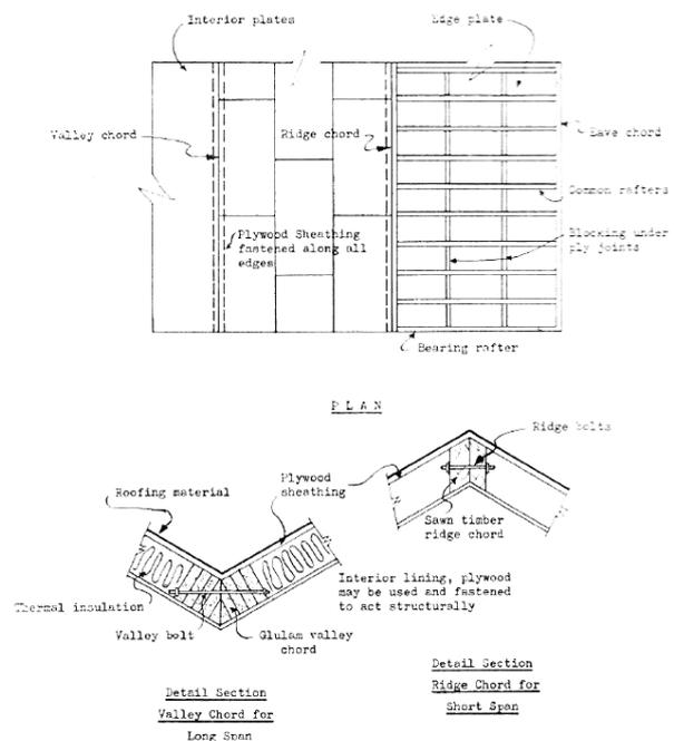
Figure 1. Folded-Plate construction detail.
