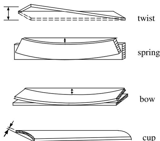
Figure 1 - Definition of different types of distortion.
