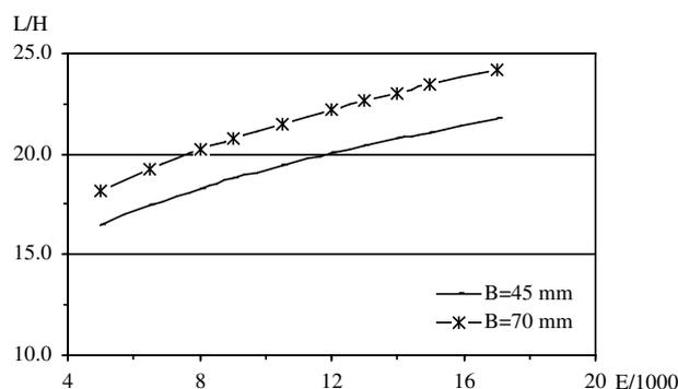
**Figure 7** - Relationship between L/H (span/height) and MOE for two different breadths (in mm) in a joist in a floor structure which fulfils the criterion of a limited deflection of 1.5 mm due to a concentrated load of 1 kN in the middle of a single span.
