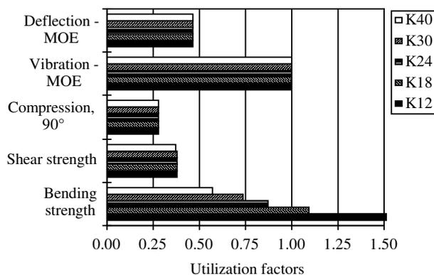
**Figure 6** - Utilization factors for floor T-joists (45 x 220 mm) with particleboard of 22 mm. Timber joists are calculated with an average E of 14 GPa independent of strength class. The span is 4.57 m for timber and 4.5 m for glulam L40 (as E = 13 GPa for glulam was taken from the Code) to obtain the same governing vibration criterion. Different characteristic bending strength applied to each structural class expressed in Kxx.
