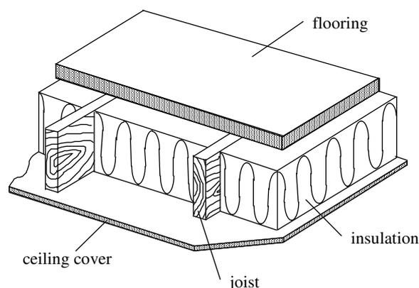
**Figure 2** - A diagrammatic sketch of a floor structure.
