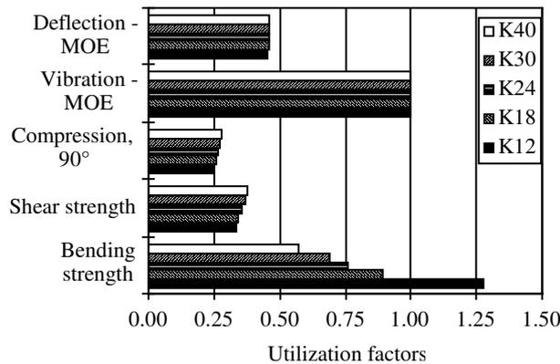
**Figure 4** - Utilization factors for floor T-joist (45 x 220 mm) with particleboard of 22 mm. The span had to vary, i.e. 4 m for K12 to 4.5 m for L40, to obtain the same governing vibration criterion. Different structural classes expressed in Kxx, where xx is the characteristic strength.
