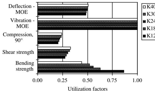
**Figure 5** - Utilization factors for floor joists (45 x 220 mm). Different structural classes expressed in Kxx, where xx is the characteristic strength. There is no interaction between particleboard and timber joist.
