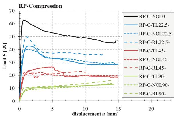
Figure 6. Load-displacement behaviour for Radiata Pine for all configurations A
