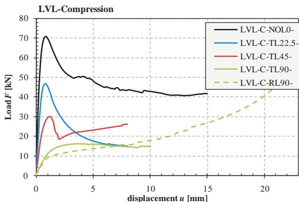
Figure 7. Load-displacement behaviour for LVL for all configurations A
