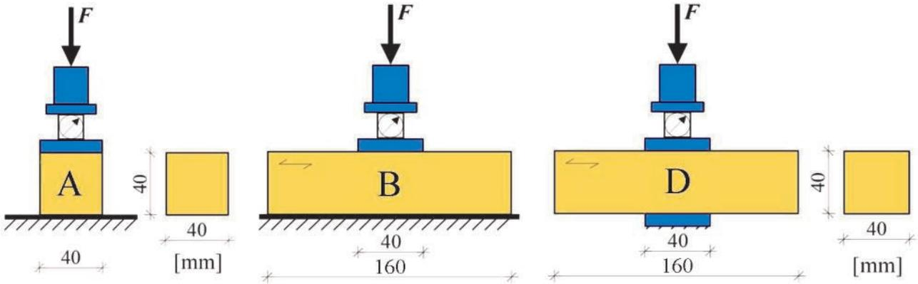
Figure 5. Test setup of the configurations A, B and D
