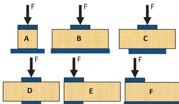
Figure 1. Loading configurations for determining compression perpendicular to grain, cf. Larsen et al. [6]
