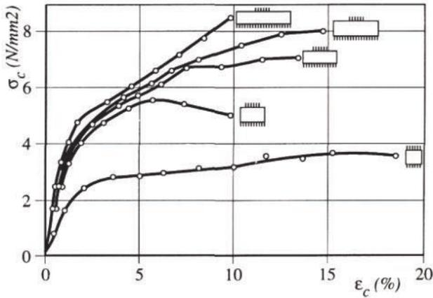
Figure 2. Different stress-strain behaviours under compression perp. to grain, cf. Suenson [14]
