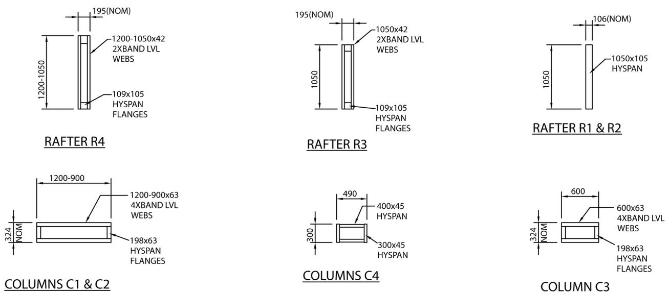
Figure 3. Rafter and Column Sections
