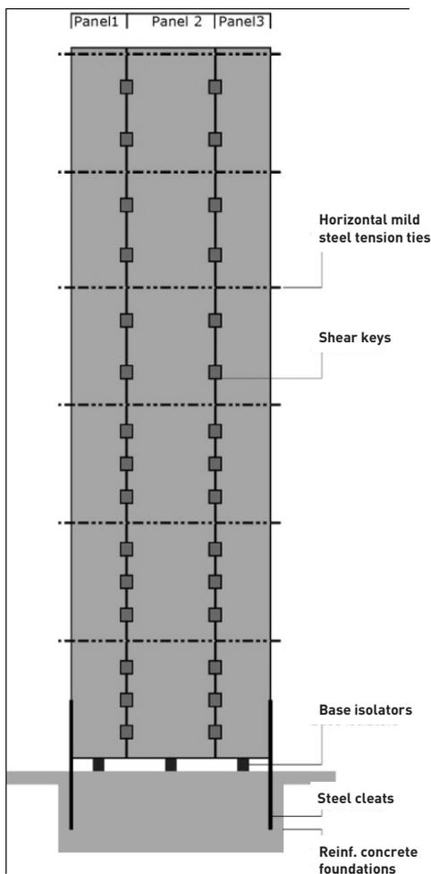
Figure 5. Elevation of 'shear wall' LLRS (diagrammatic)
