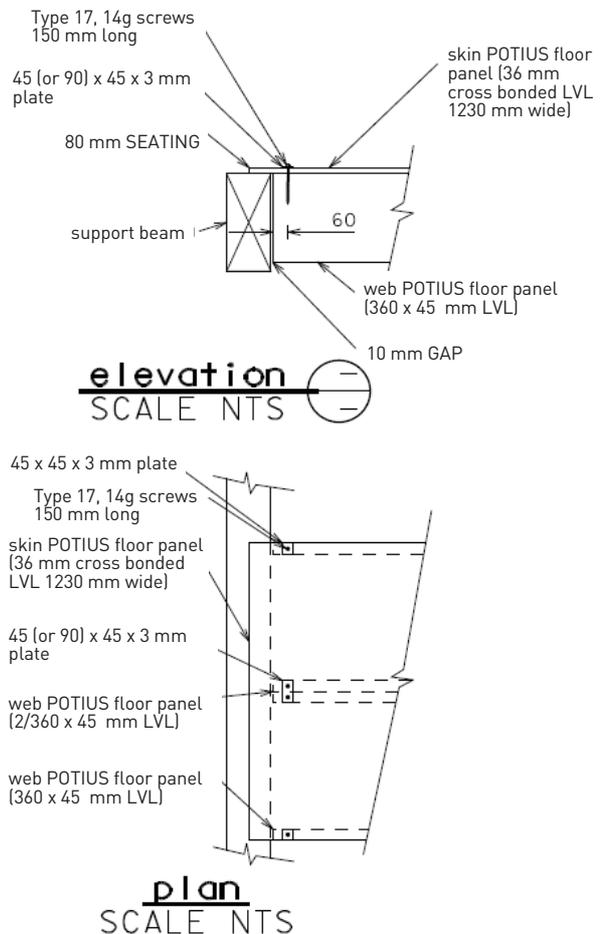
**Figure 1. Flange hung panel system.**
