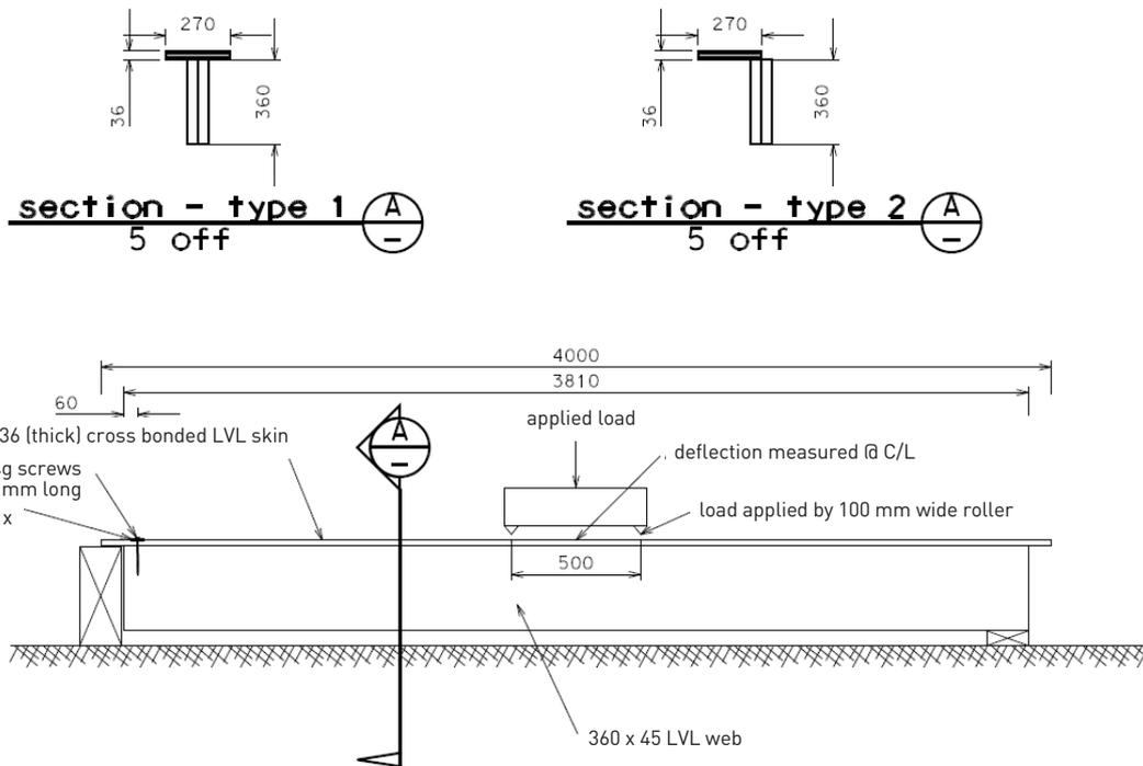
Figure 2. Proposed testing configuration
