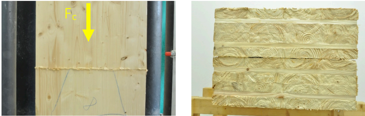
Figure 10: Typical compression failure at contact joint in CLT specimen: joint after failure (left), contact surfaces with mutual imprints of annual rings (right).
