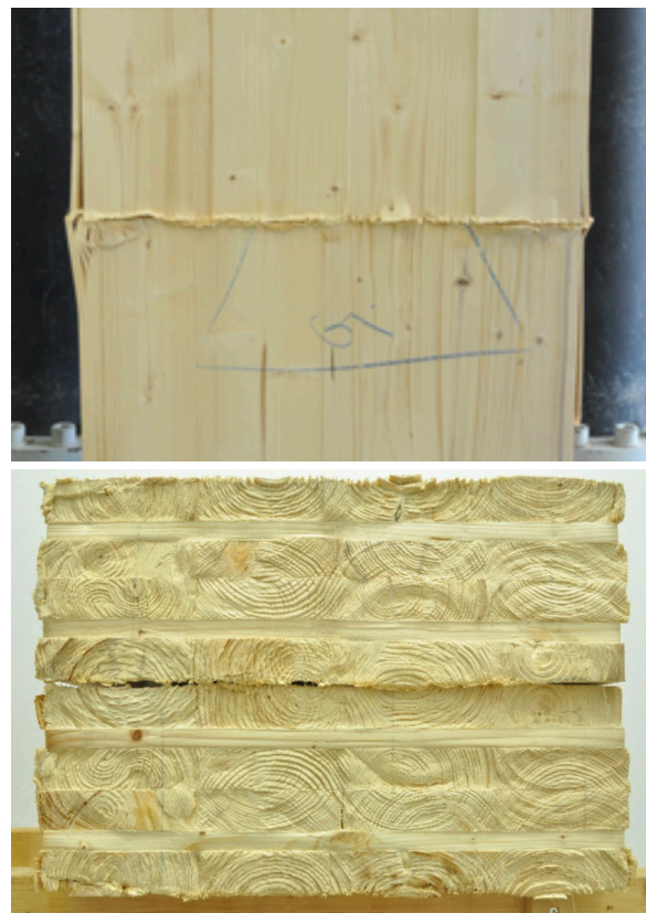
Figure 1: Typical compression failure at end grain contact joint in CLT: joint after failure (top), contact surfaces with mutual imprints of annual rings (below).
