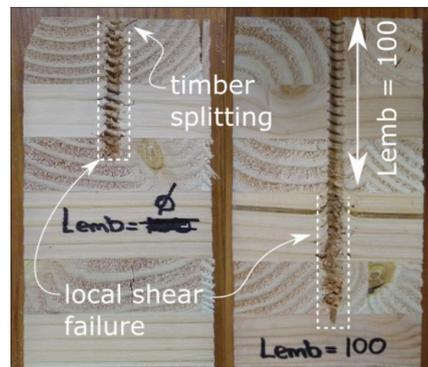
Figure 12: Comparison of  $l_{emb} = 0$  and 100mm.
