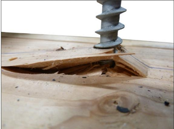
Figure 8: Timber splitting in CLT wide face 90° screw withdrawal test.
