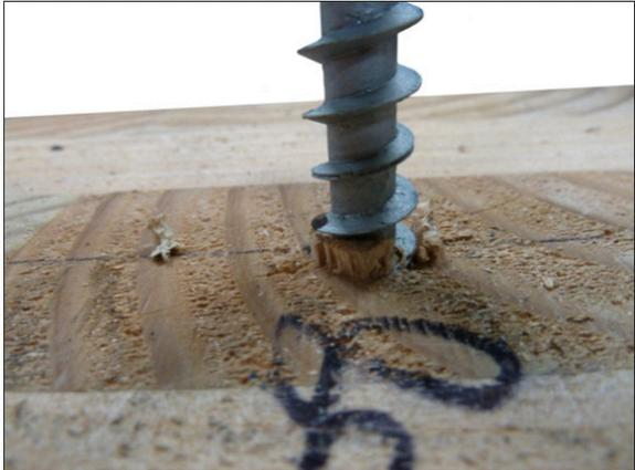
Figure 9: Shear cylinder failure in CLT narrow face 0° screw withdrawal test.
