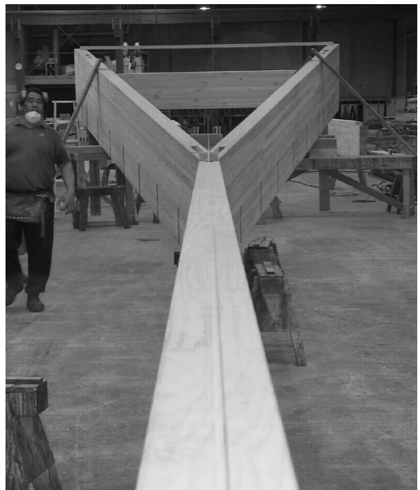
The requirement for concealed joints was achieved with insert plugs covering the edge of the slotted in steel plates.
