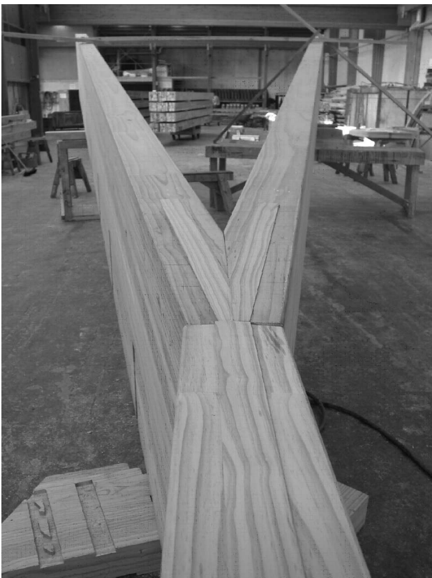
The requirement for concealed joints was achieved with insert plugs covering the edge of the slotted in steel plates.
