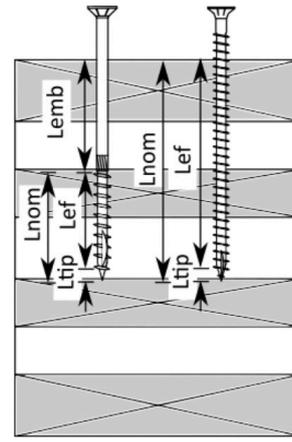
Figure 2: STS key parameters (partially threaded vs. fully threaded)
