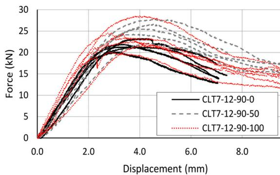
Figure 11:  $l_{emb}$  test series load-slip curves.
