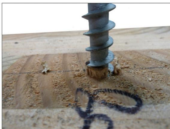
Figure 9: Shear cylinder failure in CLT narrow face  $0^\circ$  screw withdrawal test.
