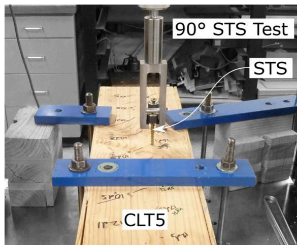
Figure 5: 90 degree screw withdrawal test setup.
