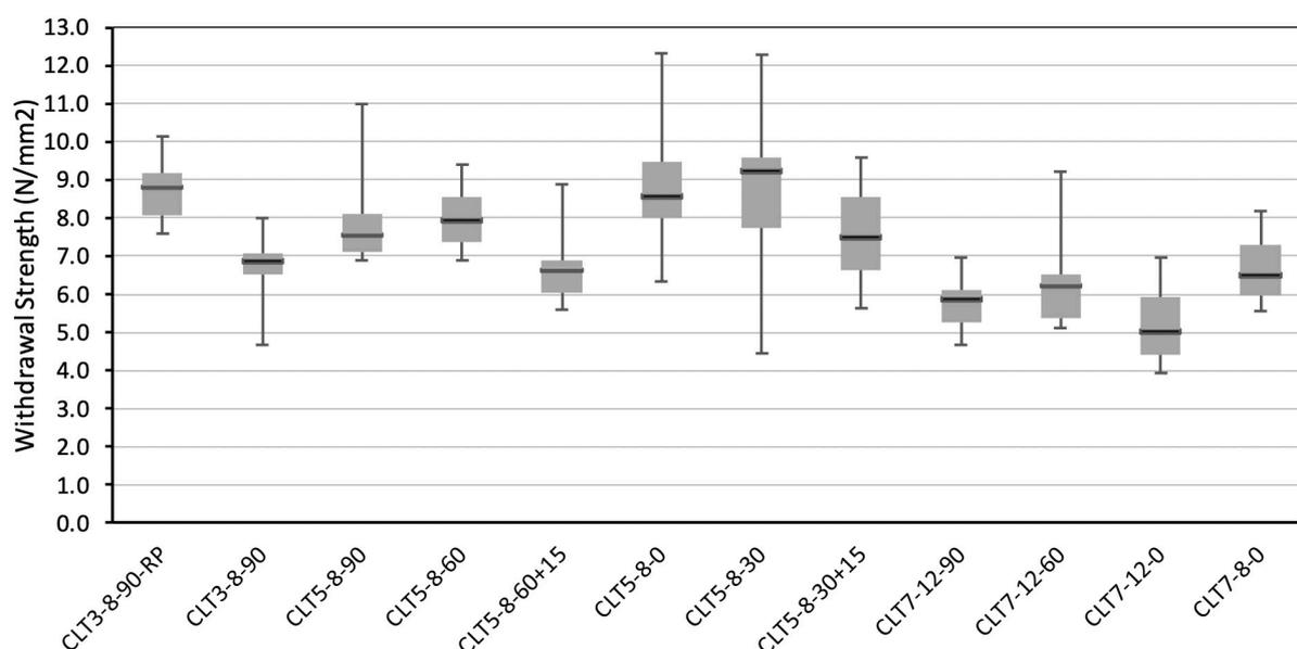
Figure 7: Withdrawal strength of various test series.
