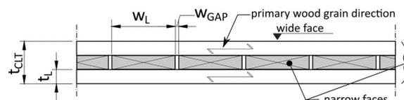
Figure 1: CLT layout with definitions.
