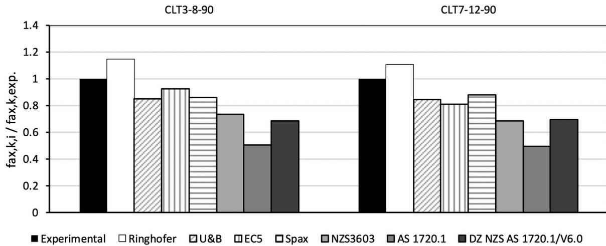
Figure 10: Comparison of characteristic withdrawal strength according to experimental results for Ø8mm and Ø12mm screws at constant 10d length and 90° installation.
