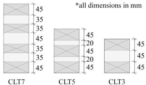
Figure 3: CLT types used in test programme.
