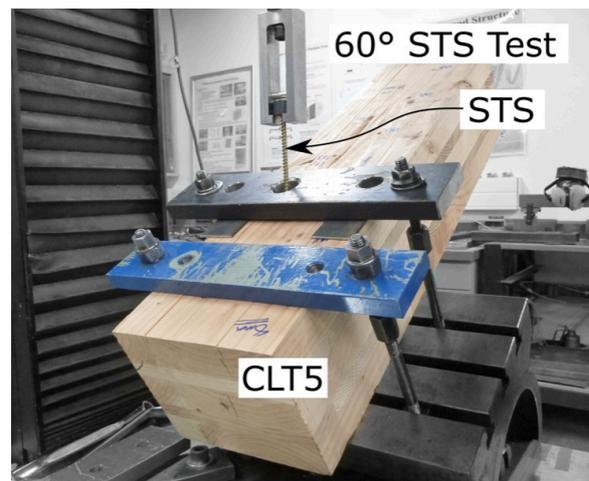
Figure 6: Inclined screw withdrawal test setup.
