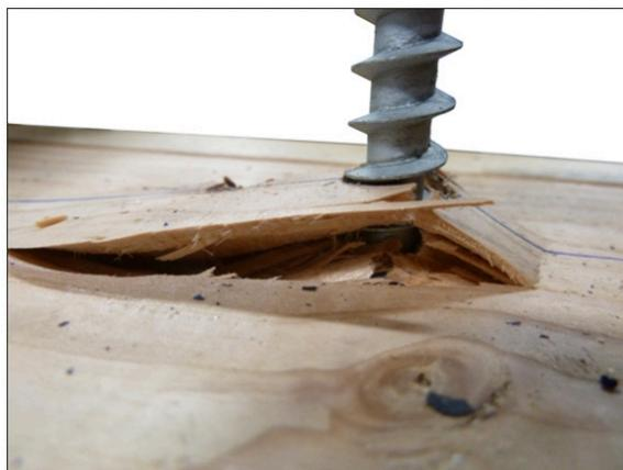
Figure 8: Timber splitting in CLT wide face  $90^\circ$  screw withdrawal test.
