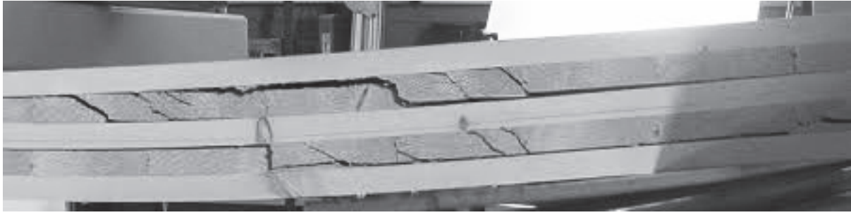
Figure 3. Shear in a generic timber section/cube. Longitudinal shear (a) and rolling shear (b).
