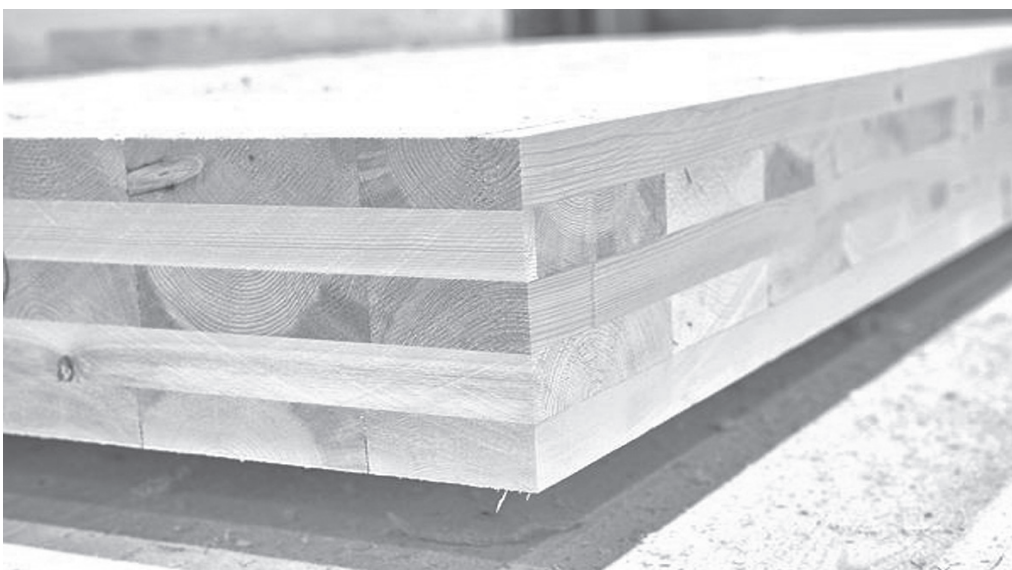
Figure 1. Cross Laminated Timber panel cross-section.
