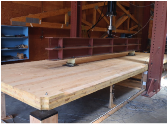
Figure 4: Point Supported CLT Panel Testing Apparatus and Failure.
