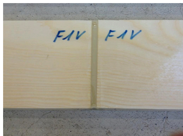
Figure 13: Butt-joint bonding of lamellas [6].
