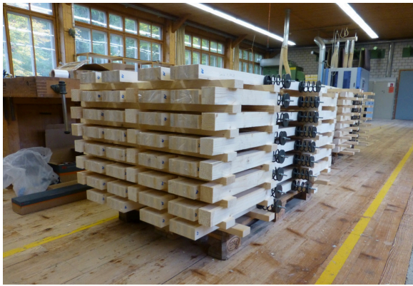
Figure 19: Long-term load bending tests on CLT-beams with bonded butt joint in the middle span of the specimen.
