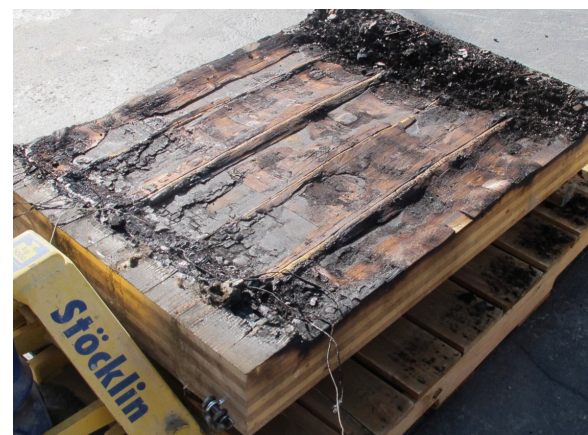
Figure 21: Small-scale fire test on spruce CLT-plate after removing the char layer.
