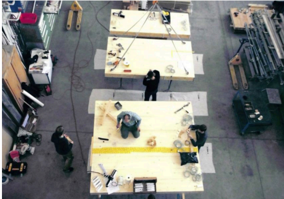
Figure 22: Bonding of CLT elements for the large-scale fire test.
