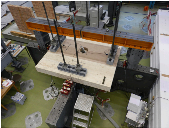
Figure 9: Testing a central slab element at ETH Zurich.
