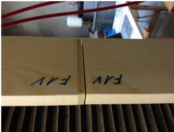
Figure 14: Butt-joint bonding of lamellas while testing [6].
