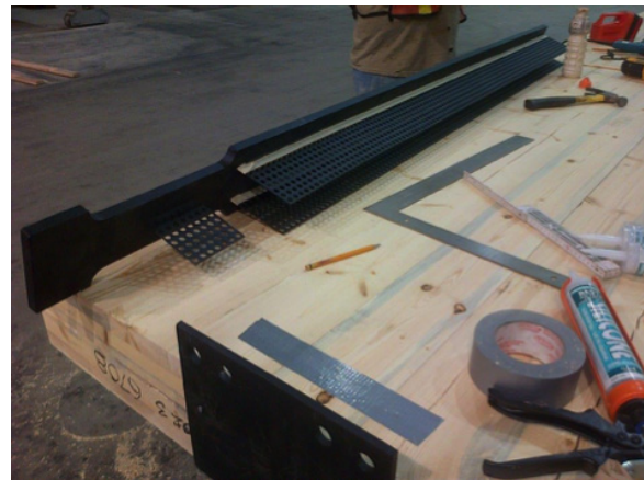
Figure 7: Typical hold down with the reduced section plate and HSK connectors.
