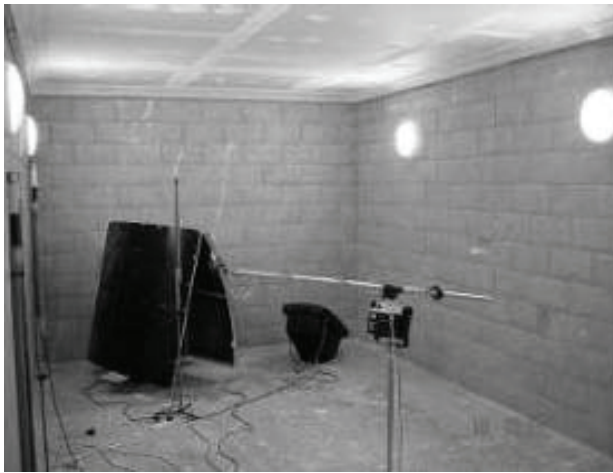
Figure 2. FloorTest Rig, End dia. pole @ 600mm centres. Measuring the sound field .
