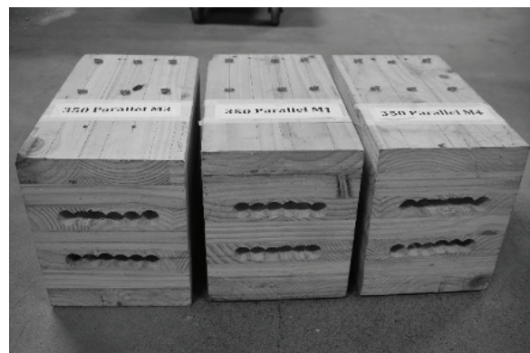
Figure 4. bottom view of CLT specimens containing M24 rods with 350 mm embedment length in the parallel to the grain lamination tested in compression.
