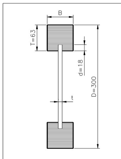
**Figure 1.** Cross-section of the I-beams
