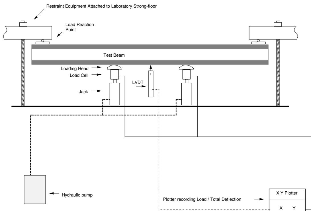
**Figure 2. Third-point loading arrangement**
