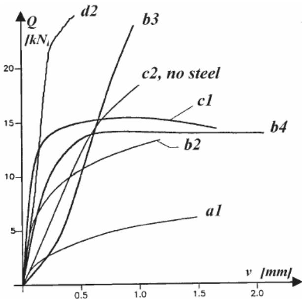
Figure 2: Schematic of load-slip behaviour of types of connection [8].
