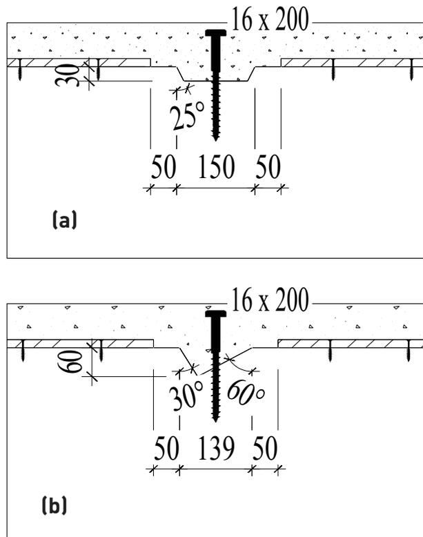
Figure 3: Notched connections – trapezoidal (a) and triangular (b) shapes (12 and 16 mm coach screw are used for 45 and 63 mm thick LVL beams respectively).
