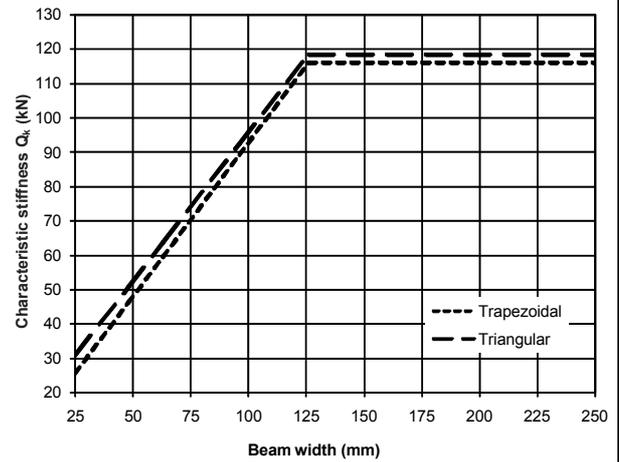
**Figure 6: Characteristic strength ( $Q_k$ ) of trapezoidal and triangular notches.**
