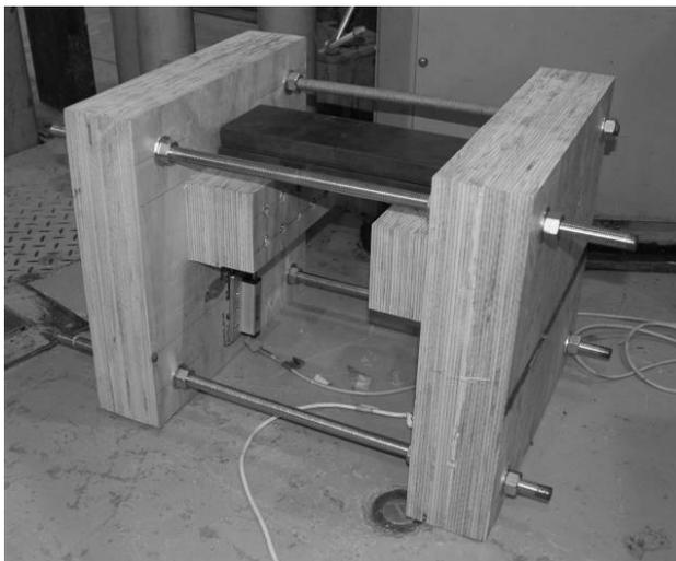
Figure 7. Corbel testing specimen for Configuration 1C.
