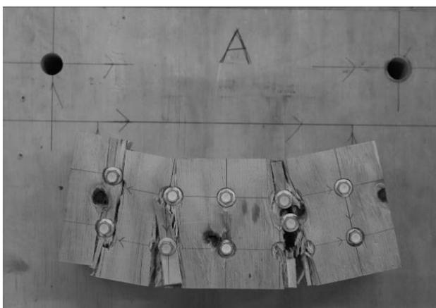
Figure 9. Corbel damage after testing of a Configuration 1A specimen with the applied load parallel to the grain of the corbel.
