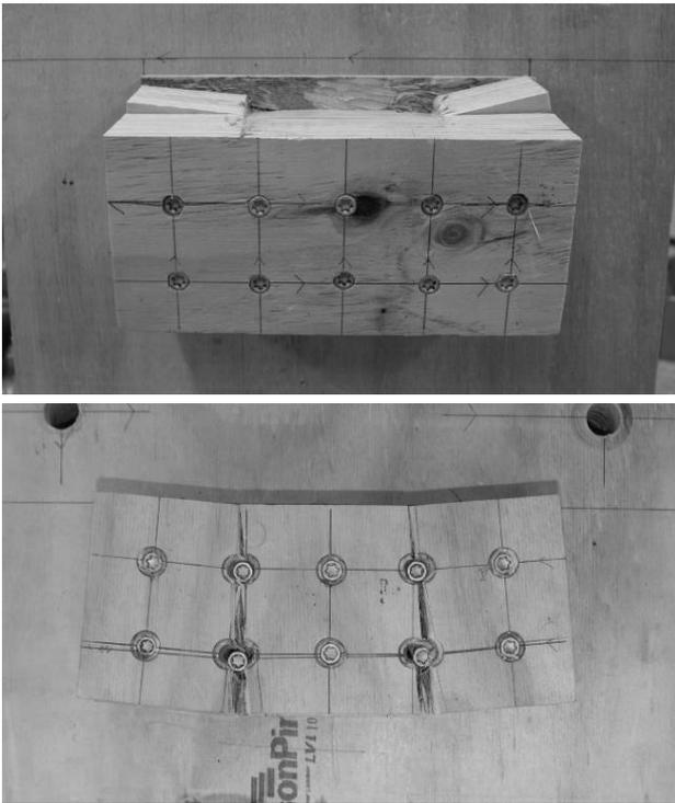
**Figure 10. Corbels following testing using SFS screws for Configuration 1C (Bottom) and 1D (Top) specimens.**
