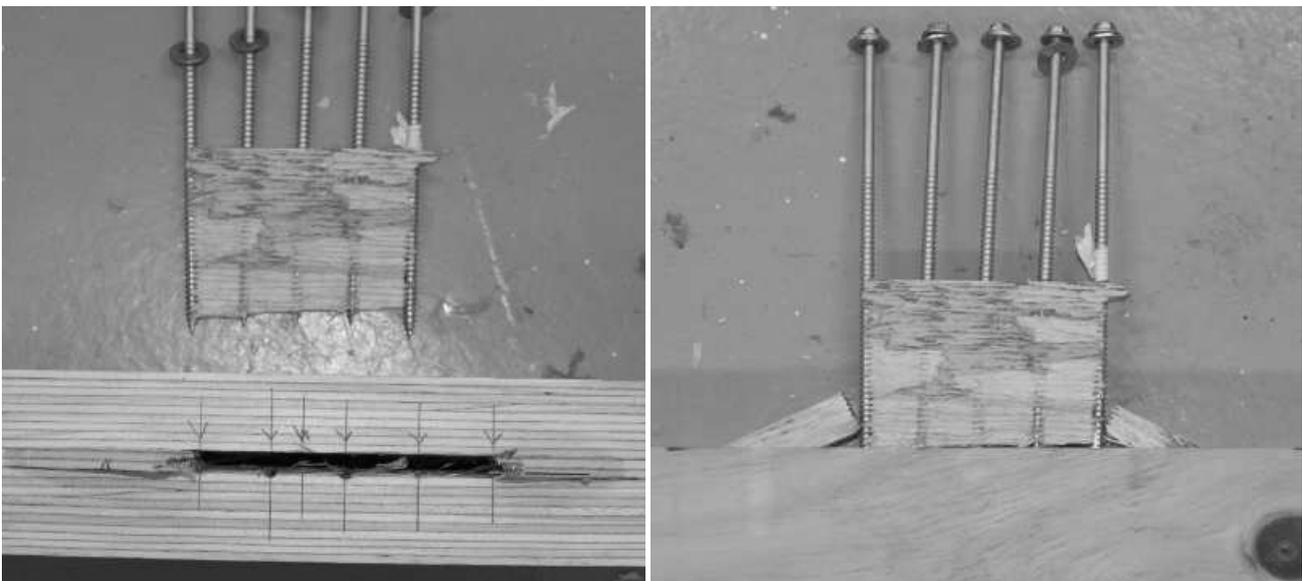
Figure 8. Shear plug failures observed during screw withdrawal tests from LVL.
