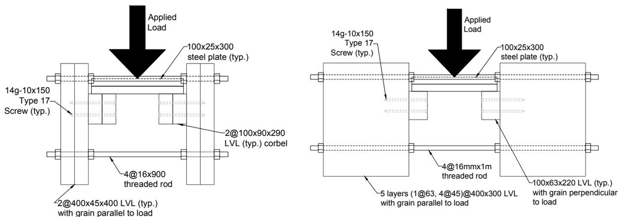
Figure 6. Corbel testing specimen example for Configurations 1 through 3 (left) and Configuration 4 (right).
