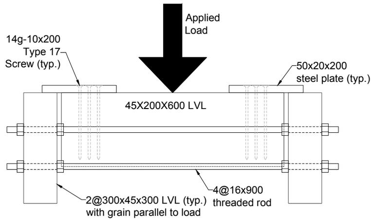
Figure 3. LVL connection testing configuration.
