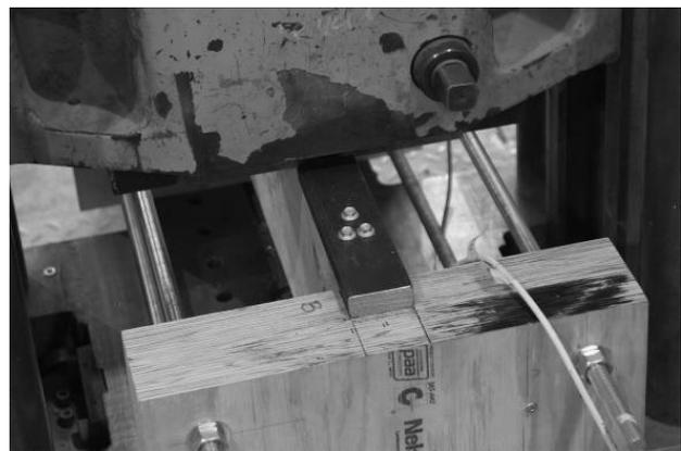
Figure 4. LVL test connection Configuration 1A.
