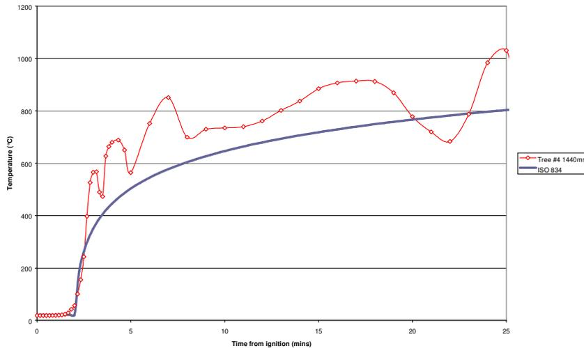
**Figure 3:** Standard furnace test temperatures compared with a compartment fire
