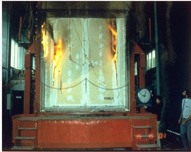
*Figure 1: Standard furnace test*
