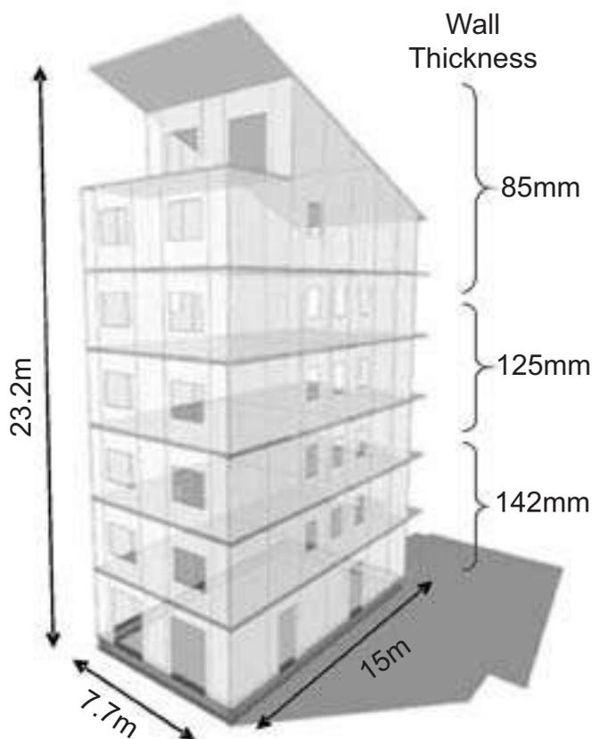
Figure 8. Seven storey cross-laminated test building dimensions and wall thicknesses.
