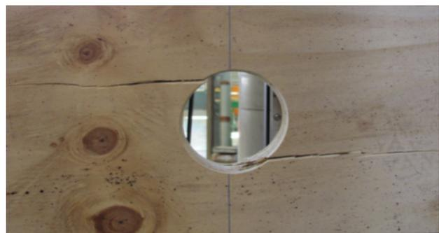
Figure 1. Crack propagation around a hole .
