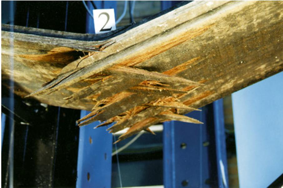
*Figure 3 - Typical failure pattern of azobé boards.*
