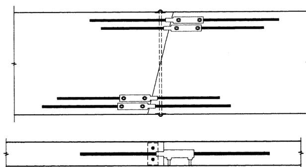
**Figure 9** Epoxy Grouted Reid Bar & Coupler
