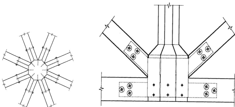
**Figure 5** Multi-Member Bolted Joint
