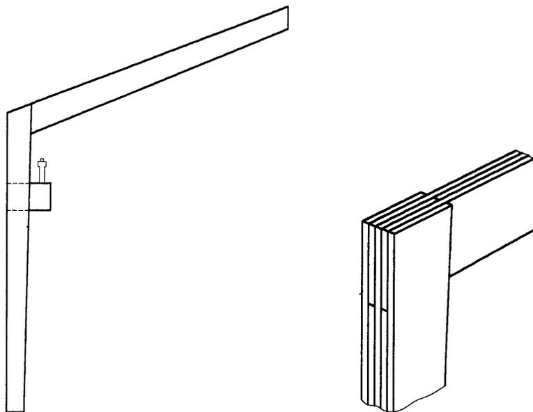
**Figure 7** Glued Cross-Lapped Joint
