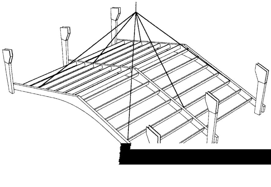
**Figure 4** Portal Frame Erection Method
