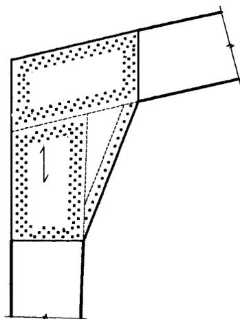
Figure 1 Nailed Plywood Gusset
