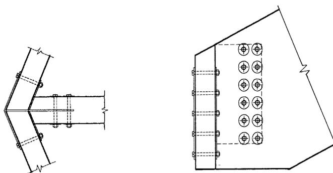
**Figure 6** Bolted Rafter to Tie Beam Connection
