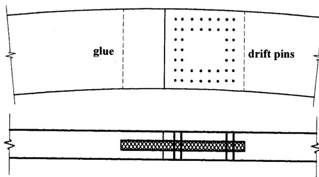
Figure 10 Timber & Drift Pin Connection
