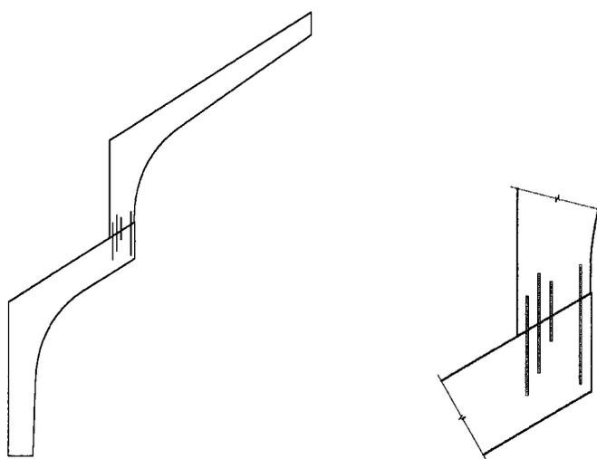
**Figure 8** Epoxy Grouted Threaded Rods
