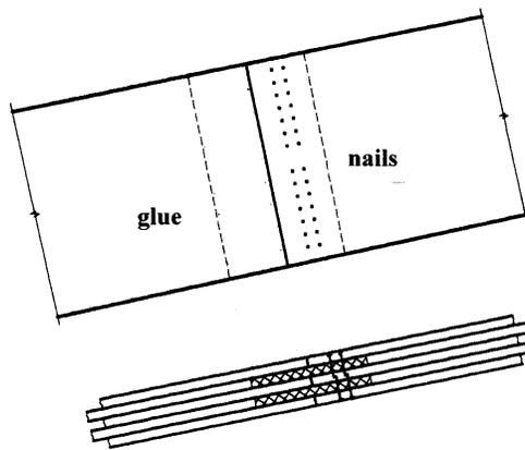
**Figure 3** Nailed Timber Splice Joint
