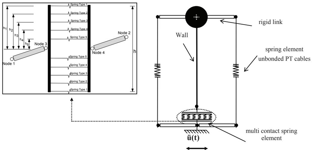
Figure 7. Schematic of multi spring model of wall.
