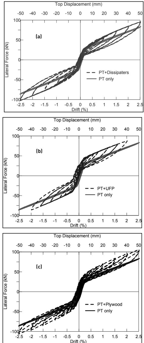
**Figure 4. Force-displacement plots of Specimens HY (a), HU (b) and HP (c) compared to Specimen PT.**
