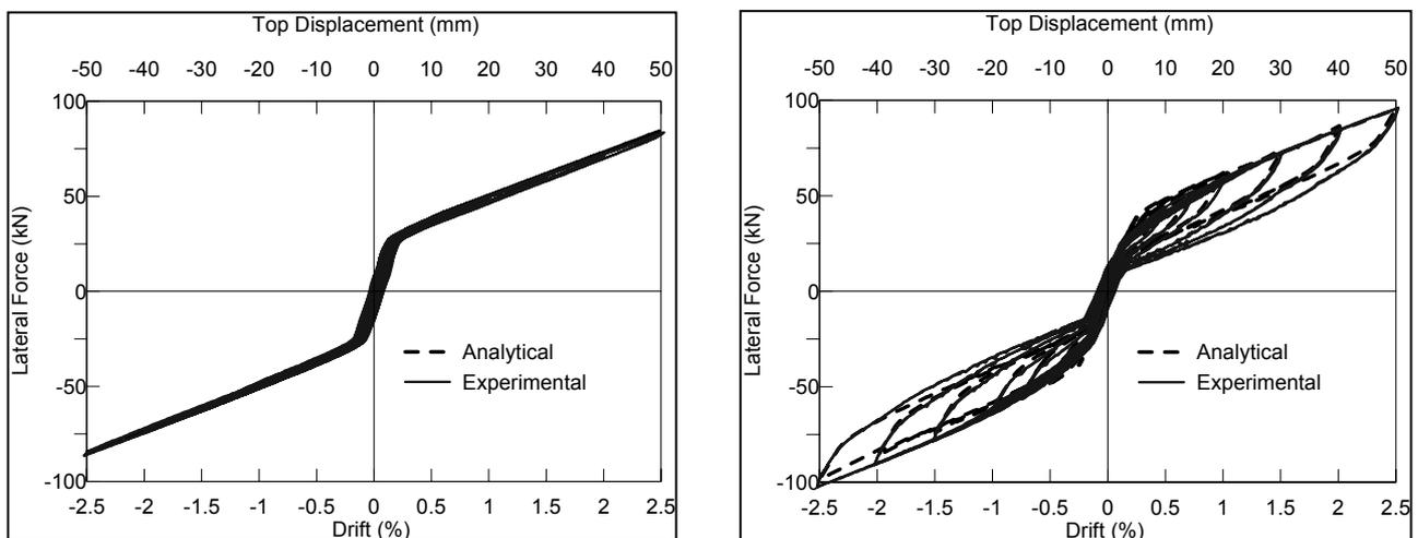
Figure 9. Force-displacement comparisons of Specimens PT (left) and HY (right).
