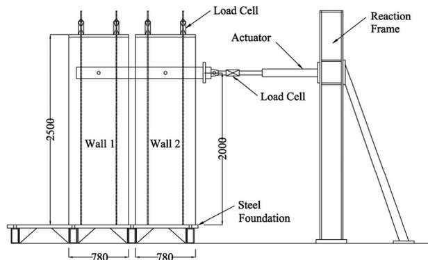
**Figure 3. General test setup of walls (dimensions in mm).**
