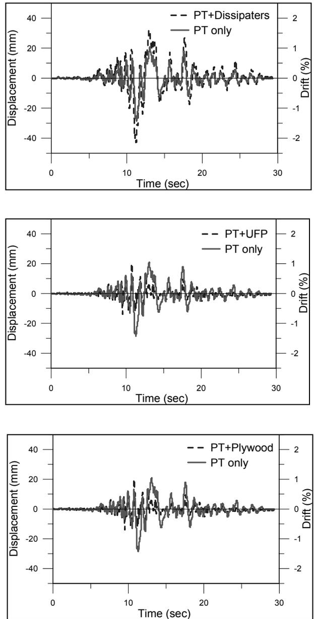
Figure 6. Time-history plots of top wall displacement for Specimens HY, HU and HP (top to bottom) compared to Specimen PT.
