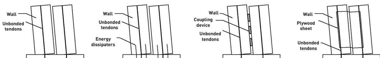
Figure 2. Post-tensioned rocking walls, post-tensioned hybrid walls and post-tensioned coupled walls.
