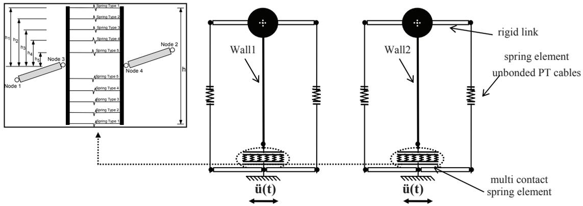
Figure 8. Schematic of multi spring model of coupled walls.
