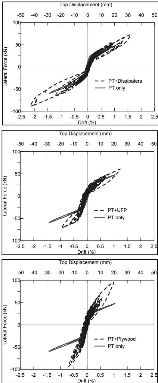
Figure 5. Pseudo-dynamic plots of Specimens HY, HU and HP (top to bottom) compared to Specimen PT.
