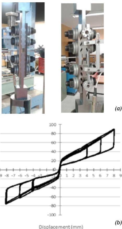
**Figure 3:** Experimental test of a double acting RSF joint a) Test setup b) Hysteresis loops
