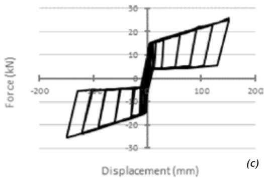
Figure 5: Numerical analysis of CLT wall with RSF joints a) Numerical model b) Loading regime c) Force-displacement loops
