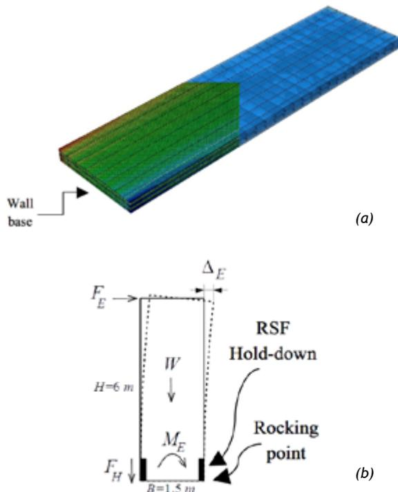
Figure 4: Numerical modelling of a CLT wall a) Assembly and stress distribution b) Elastic deflection of the wall
