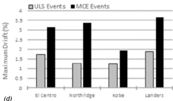
**Figure 6:** Numerical analysis of the CLT core with RSF joints a) Numerical model b) slotted plate ductile link c) Maximum lateral drifts d) Peak roof accelerations
