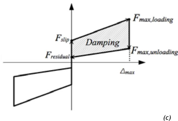
**Figure 2:** Schematic illustration of the symmetric RSF joint: a) Friction plates before slip b) Friction plates at ultimate deflection c) Schematic hysteresis loop
