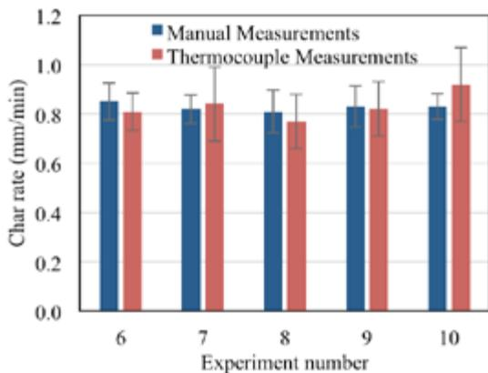
Figure 6: Comparison between manual and thermocouple char rate measurements.
