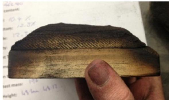
Figure 2: The edge effect on small samples of charred CLT, McTavish and Palmer [7].
