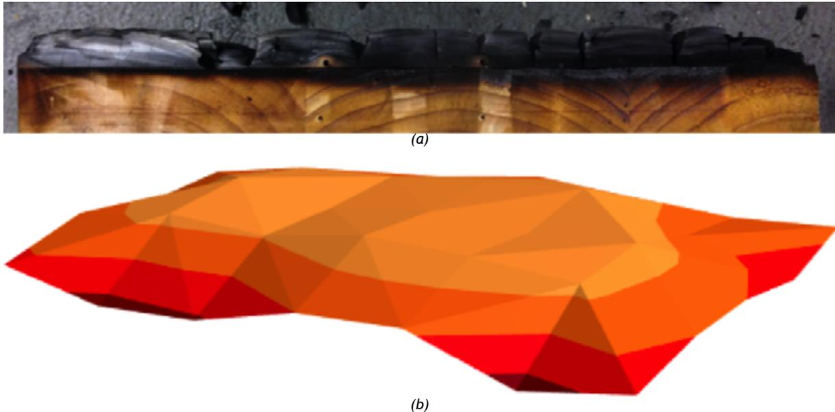
**Figure 8:** Typical char profile of sample (a) photograph before removing the char layer, showing the non-linear edge char, (b) surface plot of sample from Experiment 8 showing rounded edges.
