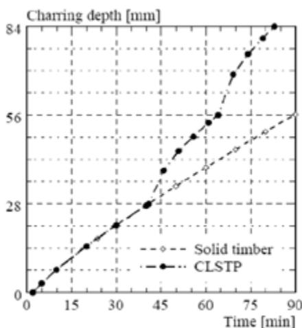
Figure 1: Charring depth with time of a CLT panel (CLSTP) consisting of 28 mm thick layers compared with solid timber, Frangi et al. [2].
