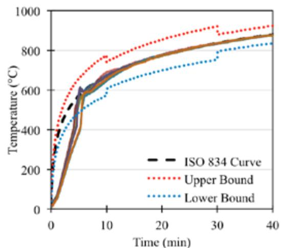
Figure 4: Furnace time temperature curves with ISO 834 curve and tolerances overlaid.
