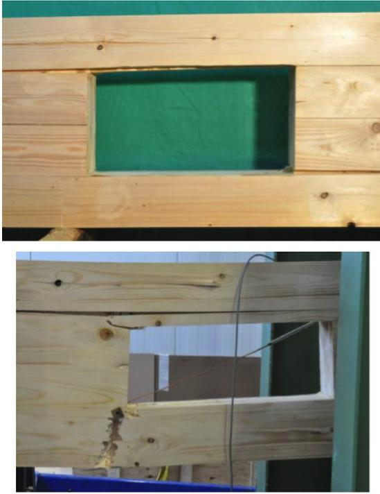
Figure 7: Shear failure in the crossing areas in specimen H50-4 (top), bending failure in the residual cross section below the hole in specimen H40-1 (bottom).
