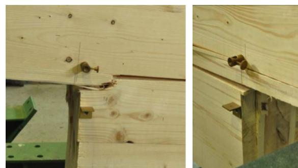
Figure 9: Shear failure in the crossing areas next to the corner of the notch.
