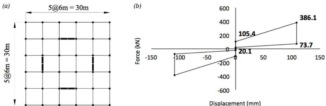
Figure 5: The prototype building: (a) Plan view (b) RSF ductile link design.
