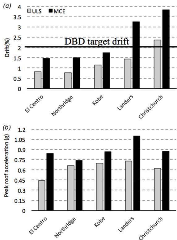
Figure 7: Numerical results: (a) Maximum lateral drifts (b) Peak roof accelerations
