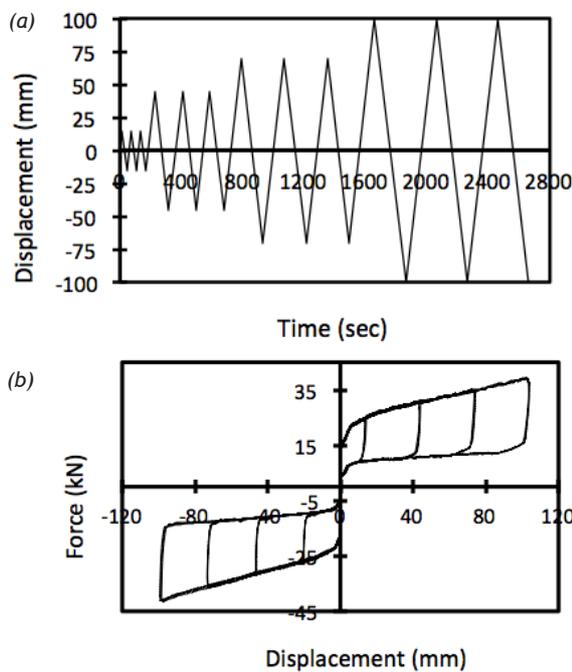
Figure 3: Test results: (a) Applied load-schedule (b) Load-deformation behaviour.
