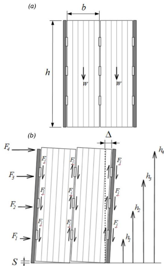
Figure 4: Rocking CLT walls coupled with RSF joints: (a) Before rocking (c) After rocking.
