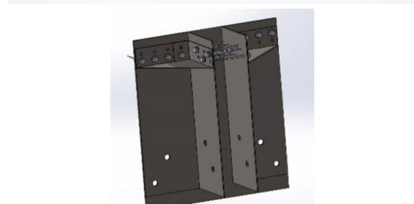
Figure 6: Sheet steel plates and brackets to join minor lateral trusses to major longitudinal truss.
