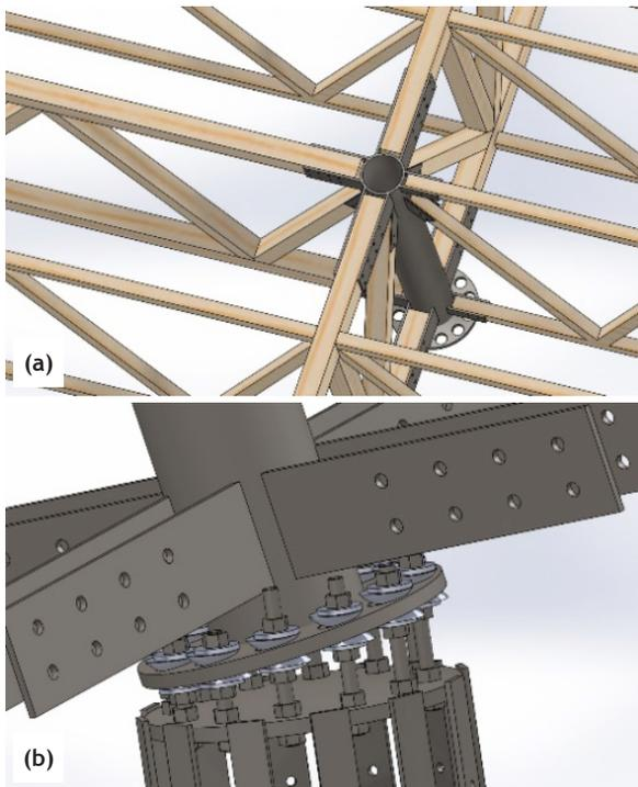
Figure 3: (a) General arrangement for moment-resisting connection between leg and trusses. (b) Spherical washer detail.
