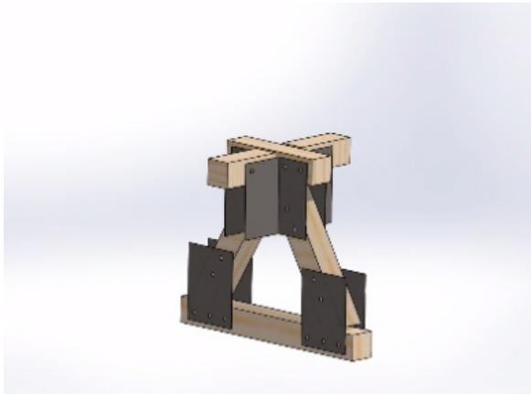
Figure 5: Test assembly for steel plate joints.
