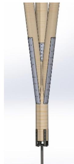
Figure 4: Joints at bottom of trunk and branch design. Three-hole straps at base were replaced with a five-hole design.
