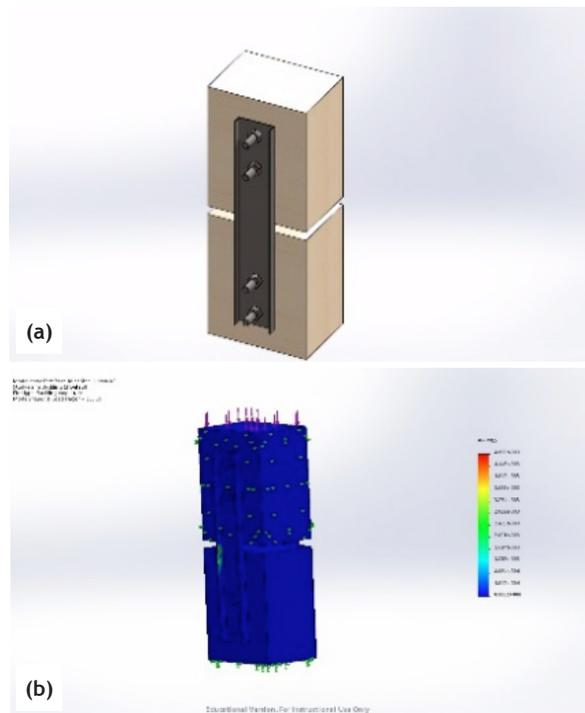
**Figure 7:** (a) Test piece for channel section splicing chords. (b) the computer-aided drawing program included a finite element post-processor which was used to choose thickness of channel, later verified by physical test. End gaps were deliberately provided in all compression test assemblies, to simulate along-grain shrinkage of timber.
