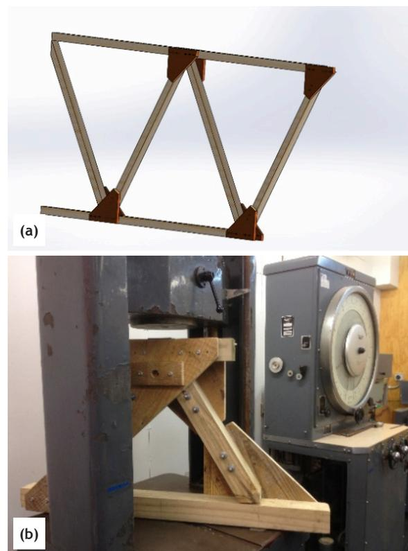
**Figure 8:** (a) Timber cheek plates (truncated triangles) on minor lateral trusses. (b) Test assembly showing crack-suppressing cleat parallel to and below chord.
