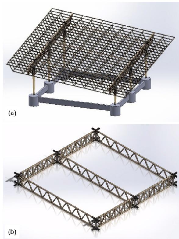
Figure 1: (a) Timber structure on buried concrete foundation. (b) Main frame comprises two longitudinal and three lateral trusses.
